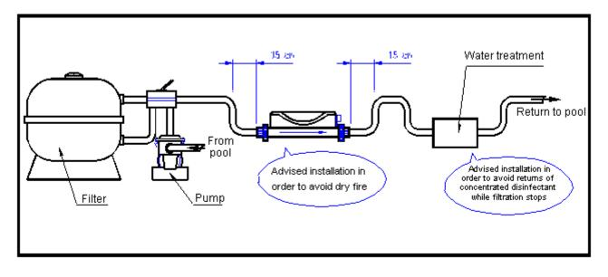
**Direction of circulation:** The direction of water circulation shall be accordingly to the arrow located on the housing of the appliance.
