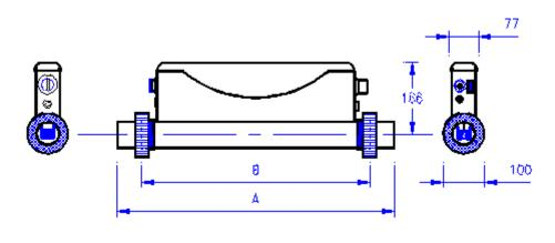
$\begin{array}{l} B \ (mm) = 452 \ RED \ LINE \ 3 \ and \ 6 \ kW \\ B \ (mm) = 552 \ RED \ LINE \ 9 \ and \ 12 \ kW \\ A \ (mm) = 538 \ RED \ LINE \ 3 \ and \ 6 \ kW \\ A \ (mm) = 638 \ RED \ LINE \ 9 \ and \ 12 \ kW \\ \end{array}$
